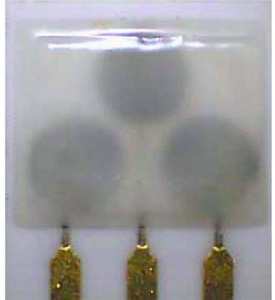
The Reference Electrode is isolated and maintains the base potential to stabilise the sensor output, even when the sensor is exposed to high concentrations of Hydrogen. Three electrode sensors have a wider detection range with good direct linearity.
