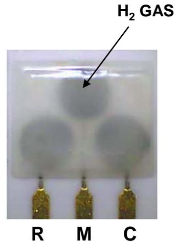
A RAW single sensor is part of a wafer which contains 48 RAW Sensors. Single RAW sensors or a complete wafer can be purchased. Every wafer is gas tested prior to shipment.
