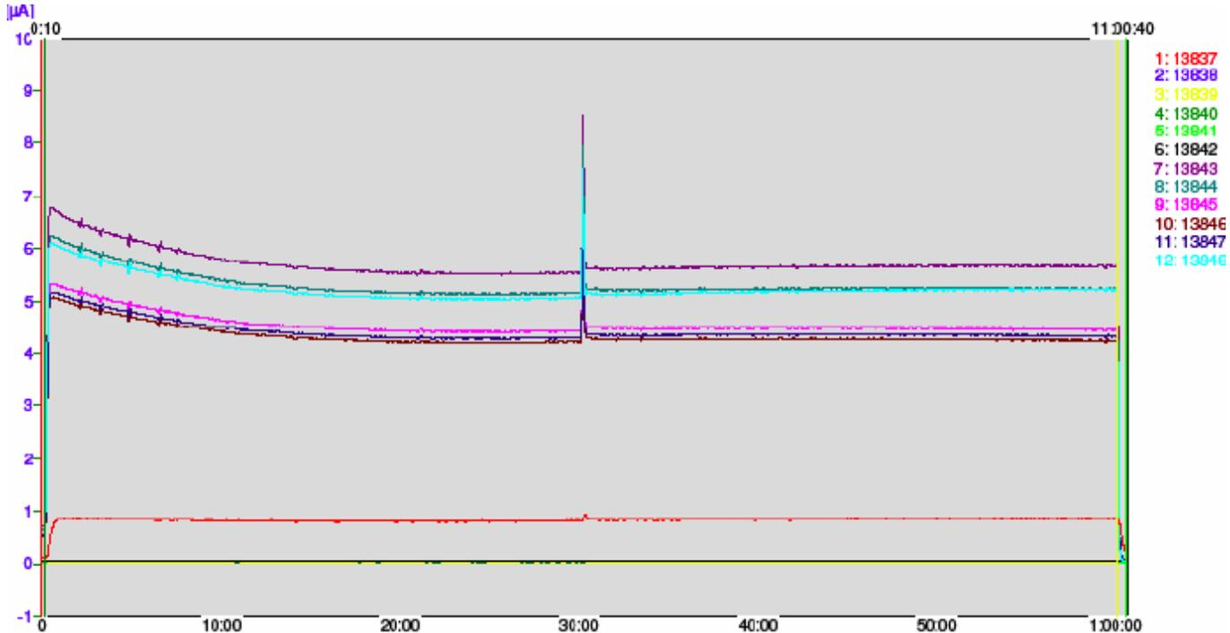
The gas concentration was 1300ppm H<sub>2</sub> and the test was conducted at room temperature of ~23°C. There is a drop of signal during the first 10 minutes due to stabilisation to the dry air. The switch to 90% RH shows no change.
