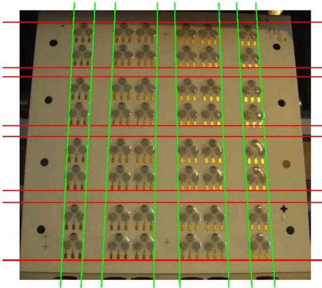
If ordering a wafer of 48 RAW sensors, it is important to break the sensors away from the wafer in the following order. The separation process is very easy if this order is followed:
