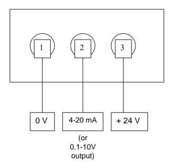
For the connection between the infrared sensor and Controller, a four wire screened cable with a total loop resistance of max. 100  $\Omega$  should be used. Terminal 1 and 3 is used for power supply 24 V d.c. The measuring signal 4-20 mA or 0.1-10V is available at terminal 2.
