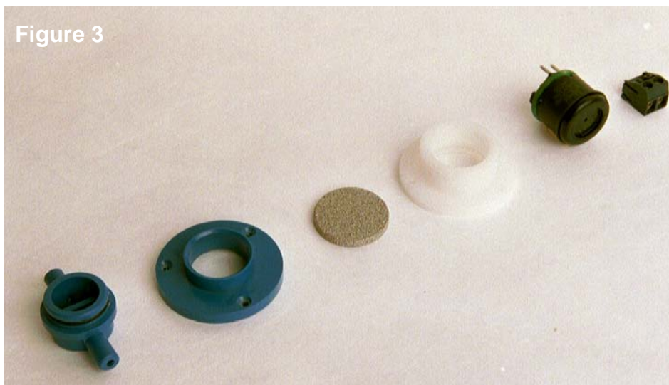
Figure 3. Components from left to right: test gas cap; installation ring; sinter metal disc; sensor holder; ECO-Sure CO sensor with O-Ring and 4-20mA transmitter; pluggable terminal block.
