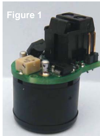
Figure 1. ECO-Sure CO sensor + 4-20mA transmitter Standard measuring range: 0-300ppm. Optional measuring range: 0-500ppm. Part no. 2112B1005
